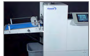
Conveyor System with Scrap Separator
