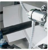
Turnover drum keeps the punched sheets in the correct page sequence and delivers them to the ejection system. Handling paperweights from 60 up to 800 gram.
